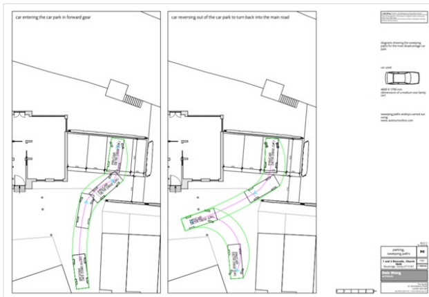
2017-0445 Unit 1 & 2 Parking Plan (showing need to reverse onto private gated land not associated with Unit 3)
